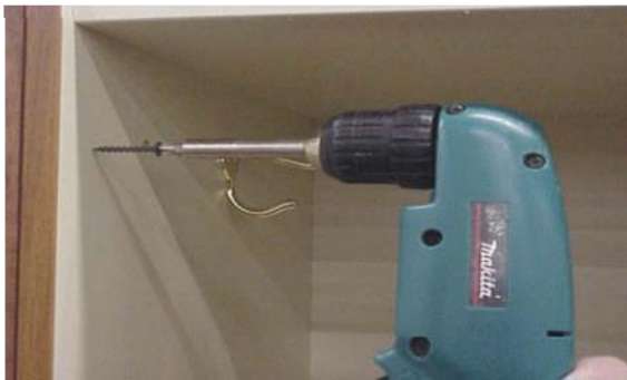
Drill drywall screw into end panel.
